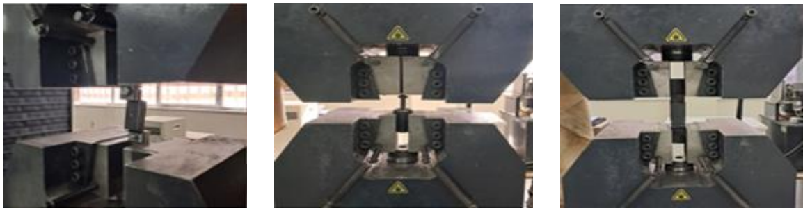
Figure 5. Test setup for dampers in universal testing machine.
